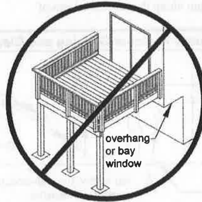
Figure 18. No Attachment to House Overhang with Ledger.
